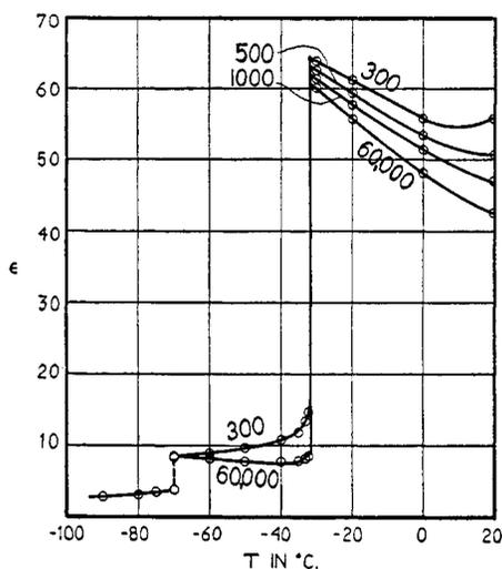
FIG. 9. Variation of the dielectric constant of dimethyl sulfate with temperature and frequency (in cycles).
