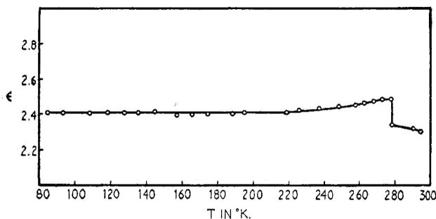
Fig. 1. Dielectric constant-temperature curve (at 50 kilocycles) of benzene
