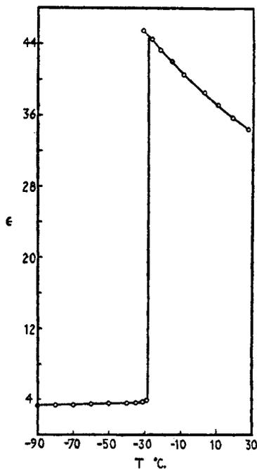
FIG. 2. Dielectric constant-temperature curve (at 70 kilocycles) of nitromethane
